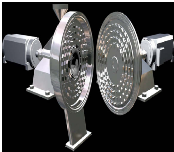
Fig. 1. Laboratory equipment for tribomechanical micronization and activation (TMA equipment).
